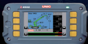
Full safe load indicator
