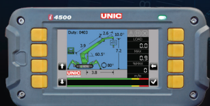
Full safe load indicator
