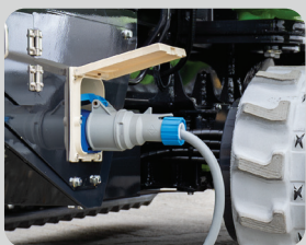
Charge the UM445 while working with a 110/240v supply
